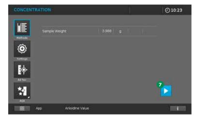
Enter the weight of the sample in grams (g), accurate to 0.001 grams (g) (5, confirm with <OK> (6, and click on <START> (7) to switch to the measurement procedure.
