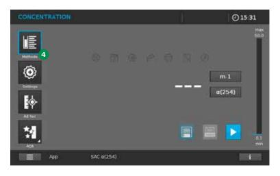
• Open the methods list (<**Methods**>) ④ and select **Method No. 300 "SAC a(254)"**.
