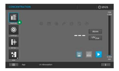
• Open the methods list (<Methods>) 4 and select Method No. 310 "UV Absorption 254".
