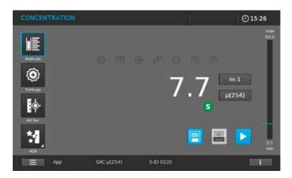
• Fill the sample solution into a corresponding rectangular quartz cell and insert the cell into the cell compartment. The measurement is performed automatically and the result appears in the display **5**.
