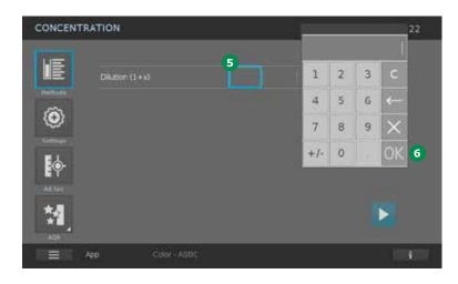
Samples with a value > 50.0 °SRM must be diluted with water. Enter the dilution factor in the proportion of 1 part sample + x parts water 5 and confirm by clicking on <OK> 6 (e.g. 1 + 9, when 10 ml of sample is mixed with 90 ml of water). If an undiluted sample is being measured, enter the value "0" and confirm with<OK> 6.
