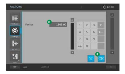
Tip on the input field "Factor" 8, enter the corrected ADMI factor, and confirm by clicking on <OK> 9.
