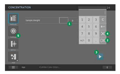
• Enter the weight of the sample in grams (g), accurate to 0.1 grams (g) 1, confirm with "OK" 2, and change to the measurement procedure by clicking on "START" 3.
