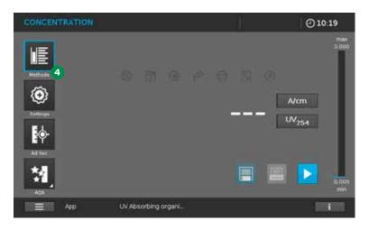
• Open the methods list (<Methods>) ④ and select Method No. 309 "UV Absorbing Organic Constituents" resp. No. 310 "UV Absorption 254".
