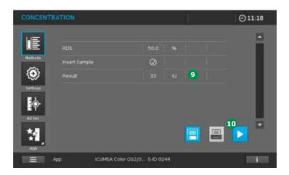
The measurement result in the units IU appears in the photometer display 9.
