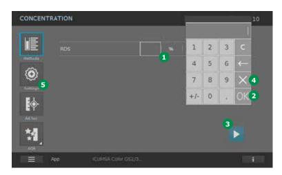
Enter the RDS factor of the sample in %, accurate to 0.1% 1, confirm with "OK" 2, and change to the measurement procedure by clicking on "START" 3.
