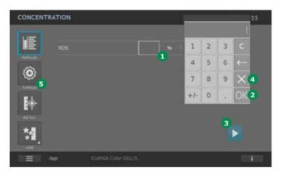
Enter the RDS factor of the sample in %, accurate to 0.1% 1, confirm with "OK" 2, and change to the measurement procedure by clicking on "START" 3.
