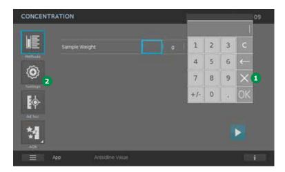
A window with an input field to enter the sample weight pops up. Close the input field without entering a sample weight by clicking on  $\langle X \rangle$  1 and click on the button  $\langle Settings \rangle$  2.
