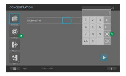
A window with an input field to enter the dilution factor pops up. Close the input field without entering a ilution factor by clicking on  $\langle X \rangle$  1 and click on the button  $\langle Settings \rangle$  2.
