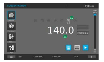
The window changes to the methods display. The activated dilution factor appears in the display 0 and is automatically taken into account in the calculation of the result 1.
