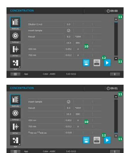
The measurement results in the units °SRM and EBC as well as the absorptions at 430 nm and 700 nm and also the quotient " $A_{700 \text{ nm}}$  /  $A_{430 \text{ nm}}$ " appear in the photometer display 10.
