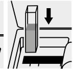
Place the cell into the cell compartment.
