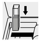
Place the cell into the cell compartment.
