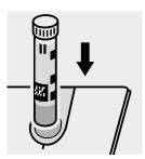
Place the cell into the cell compartment. Align the mark on the cell with that on the photometer. The measurement is performed automatically. = cell B
