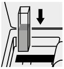
Place the cell into the cell compartment.
