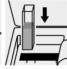
Place the cell into the cell compartment.
