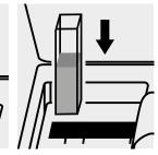
Place the cell into the cell compartment.
