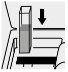
Place the cell into the cell compartment.
