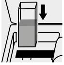
Place the cell into the cell compartment.
