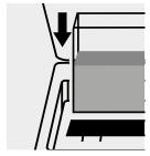
Place the cell into the cell compartment.
