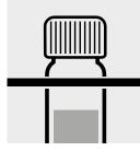
Remove the cell from the thermoreactor and place in a test-tube rack to cool to room temperature.
