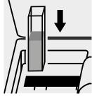
Place the cell into the cell compartment.
