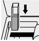
Place the cell into the cell compartment.
