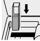
Place the cell into the cell compartment.
