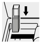
Place the cell into the cell compartment.
