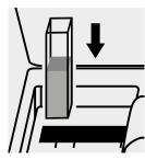
Place the cell into the cell compartment.
