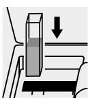
Place the cell into the cell compartment.
