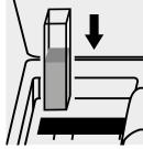
Place the cell into the cell compartment.
