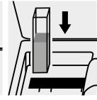
Place the cell into the cell compartment.
