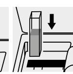
Place the cell into the cell compartment.
