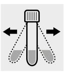
Shake the cell vigorously for 1 minute. Leave to stand to allow phases to separate.
