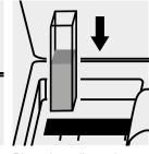
Place the cell into the cell compartment.
