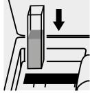
Place the cell into the cell compartment.
