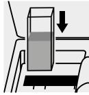
Place the cell into the cell compartment.
