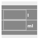
Select method no. 2509. Enter the volumes of the original sample in liters and extract (volumetric flask) in milliliters.
