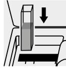
Place the cell into the cell compartment.
