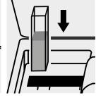
Place the cell into the cell compartment.
