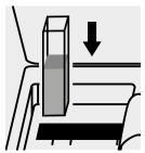
Place the cell into the cell compartment.
