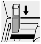
Place the cell into the cell compartment.
