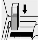
Place the cell into the cell compartment.
