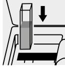
Place the cell into the cell compartment.
