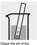
Check the pH of the sample, specified range: pH 2–10. If required, add dilute sodium hydroxide solution or hydrochloric acid drop by drop to adjust the pH.
