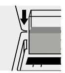
Place the cell into the cell compartment.
