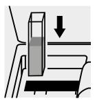
Place the cell into the cell compartment.
