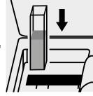
Place the cell into the cell compartment.
