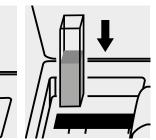
Place the cell into the cell compartment.
