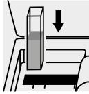
Place the cell into the cell compartment.
