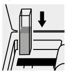
Place the cell into the cell compartment.
