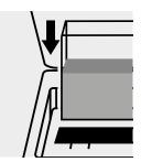
Place the cell containing the sample into the cell compartment.
