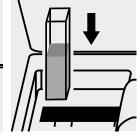
Place the cell into the cell compartment.
