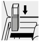
Place the cell into the cell compartment.
