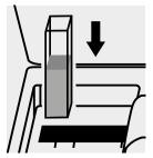
Place the cell into the cell compartment.
