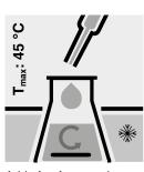
Add slowly to each Erlenmeyer flask 25 ml of Sulfuric acid for the determination of COD (Cat. No. 1.17048) with glass pipette under cooling and stirring.
