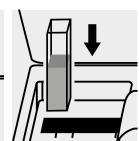
Place the cell into the cell compartment.
