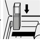
Place the cell into the cell compartment.
