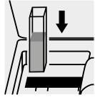
Place the cell into the cell compartment.
