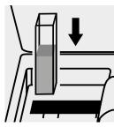
Place the cell into the cell compartment.
