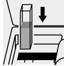
Place the cell into the cell compartment.
