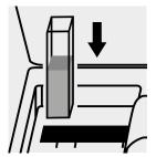
Place the cell into the cell compartment.
