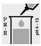
Pipette 5.0 ml of the sample into a test tube. If required, add dilute sodium hydroxide solution or sulfuric acid drop by drop to adjust the pH and bring the sample to the appropriate temperature.
