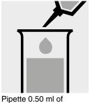
H<sub>2</sub>O<sub>2</sub>-1 into a test tube.
