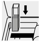
Place the cell into the cell compartment.
