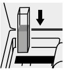
Place the cell into the cell compartment.
