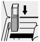
Place the cell into the cell compartment.
