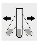
Shake the test tube vigorously to dissolve the solid substance.
