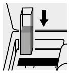
Place the cell into the cell compartment.
