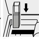
Place the cell into the cell compartment.
