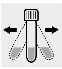
Shake both cells vigorously to dissolve the solid substance.
