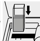
Place the cell into the cell compartment.
