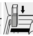
Place the cell into the cell compartment.
