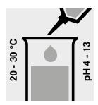
Pipette 5.0 ml of the sample into a test tube. If required, add dilute sodium hydroxide solution or sulfuric acid drop by drop to adjust the pH and bring the sample to the appropriate temperature.
