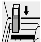
Place the cell into the cell compartment.
