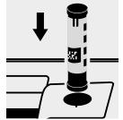
Select method with AutoSelector measuring range 2.5 – 25.0 mg/l Cl.
