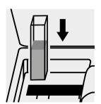
Place the cell into the cell compartment.
