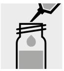
Pipette 1.0 ml of pretreated sample into a test acid. tube with screw cap.
