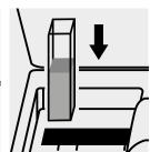
Place the cell into the cell compartment.
