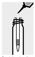
Detach the column from the reservoir. Apply 3 separate 1-ml portions of **AOX-3**. Discard the wash solution.
