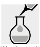
Make up the contents of the volumetric flask to the mark with distilled water (Water for analysis EMSURE®, Cat.No. 1.16754, is recommend-
