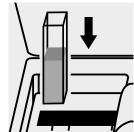
Place the cell into the cell compartment.
