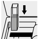
Place the cell into the cell compartment.
