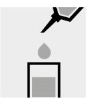
Transfer the solution into the quartz cell.
