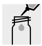
Pipette 1.0 ml of the sample into an empty round cell (Empty cells, Cat.No. 1.14724).
