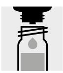
Add 3 drops of **Mg-2K**, close the cell with the screw cap and mix.
