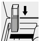
Place the cell into the cell compartment.
