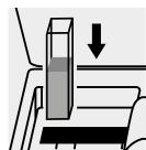
Place the cell into the cell compartment.
