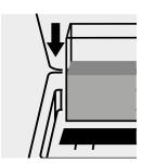
Place the cell into the cell compartment.
