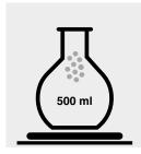
Weigh pulverized sample into a 500-ml volumetric flask, accurately weighed to 0.1 mg.
