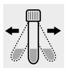
Shake the cell **vigorously for 5 seconds** to dissolve the solid substance.
