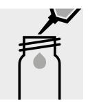
Add 9.0 ml of distilled water (Water for analysis EMSURE®, Cat.No. 1.16754, is recommended) with pipette.
