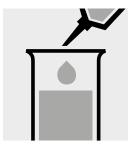
Pipette 5.0 ml of distilled water (Water for analysis EMSURE®, Cat.No. 1.16754, is recommended) into a second test tube. (Blank)
