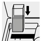
Place the cell into the cell compartment.
