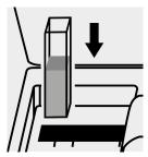
Place the cell into the cell compartment.
