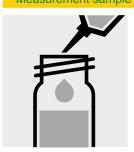
Pipette 0.100 ml of pretreated sample (filtrate) into a test tube with screw cap.
