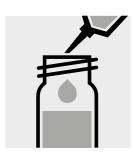
Pipette 0.50 ml of the sample into a reaction cell, **do not mix**.
