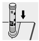
Place the cell into the cell compartment. Align the mark on the cell with that on the photometer. The measurement is performed automatically. = cell B
