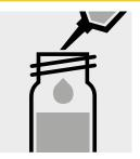
Pipette 2.0 ml of distilled water (Water for analysis EMSURE®, Cat.No. 1.16754, is recommended) into a closable vessel (20 ml).
