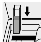
Place the cell into the cell compartment.
