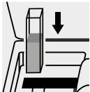
Place the cell into the cell compartment.
