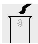
Place 1 level grey microspoon of **SO**<sub>3</sub>-1 into a dry test tube.
