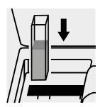
Place the cell into the cell compartment.
