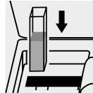
Place the cell into the cell compartment.
