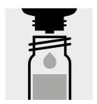
Add 3 drops of **H-2K** to the already measured cell, close the cell with the screw cap, and mix.
