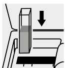
Place the cell into the cell compartment.
