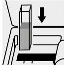
Place the cell into the cell compartment.
