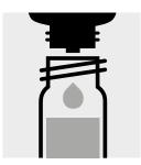
Add 3 drops of **Mn-2K**, close the cell with the screw cap, and mix.
