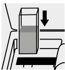
Place the cell into the cell compartment.
