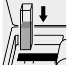
Place the cell into the cell compartment.
