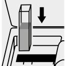
Place the cell into the cell compartment.
