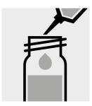
Pipette 3.0 ml of stirred sample into a reaction cell.
