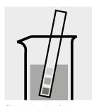
Check the pH of the sample, specified range: pH 0 – 10.
