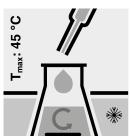
Add slowly to each Erlenmeyer flask 25 ml of Sulfuric acid for the determination of COD (Cat. No. 1.17048) with glass pipette under cooling and stirring.
