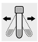
Shake the cell vigorously for 1 minute to dissolve the solid substance.
