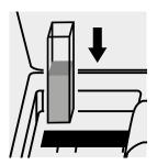
Place the cell into the cell compartment.
