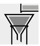
Filter the entire mixture over a hydrophobic filter acc. to ÉN 1141 [1] or §64 LFGB 31.00-7 [2]: reagent blank.
