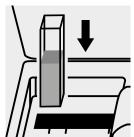
Place the cell into the cell compartment.
