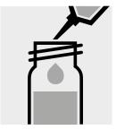
Pipette 0.50 ml of **Zn-2K** into a reaction cell, close with the screw cap, and mix.
