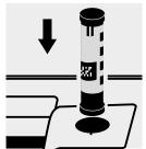
Select method with AutoSelector measuring range 0.5 – 50.0 mg/l Si.
