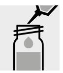
Add 0.50 ml of the sample with pipette, close the cell with the screw cap, and mix.
