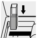
Place the cell into the cell compartment. The measurement is
