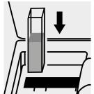
Place the cell into the cell compartment.
