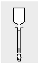
Attach the glass reservoir to the prepared column (closed at the bottom end).
