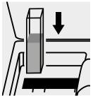
Place the cell into the cell compartment.
