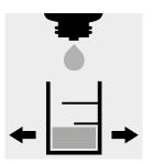
Check the chloride content of the depleted sample using MQuant® Chloride Test (Cat. No. 1.11132) according to the application (see the website): Specified value <2000 mg/l Cl<sup>-</sup>.
