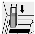
Place the cell into the cell compartment.
