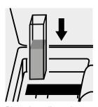
Place the cell into the cell compartment.
