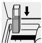
Place the cell into the cell compartment.
