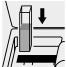
Place the cell into the cell compartment.
