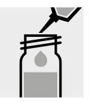
Add 5.0 ml of distilled water (Water for analysis EMSURE®, Cat.No. 1.16754, is recommended) with pipette, close with the screw cap, and
