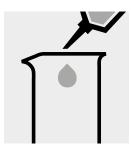
Place 20 ml of distilled water (Water for analysis EMSURE®, Cat.No. 1.16754 is recommended) into a second suitable vessel. (Blank)
