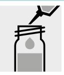
Pipette 5.0 ml of the sample into a test tube with screw cap.
