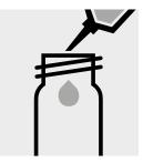
Pipette 5.0 ml of the pretreated sample into an empty round cell (Empty cells, Cat.No. 1.14724).
