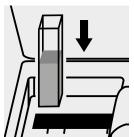
Place the cell into the cell compartment.
