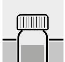
Temper the vessel in a water bath at  $95 \pm 5$  °C for **exactly** 10 minutes.
