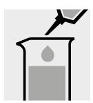
Add to each vessel 1.0 ml of **Si-3** with pipette and mix.
