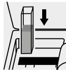
Place the cell into the cell compartment.
