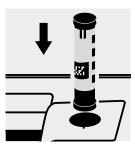
Select method with AutoSelector measuring range 0.002 - 0.100 mg/l.
