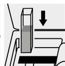
Place the cell into the cell compartment.
