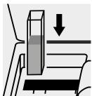
Place the cell into the cell compartment.
