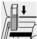
Place the cell into the cell compartment.
