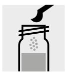
Add 1 level blue microspoon of CN-4, close the cell with the screw cap.
