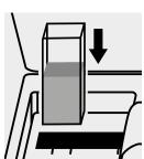
Place the cell into the cell compartment.
