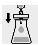
Filter or centrifuge turbid samples.
