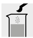
Add 1 level green microspoon of **Zn-1K** and shake to dissolve the solid substance: **sample-reagent mixture**.
