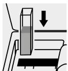
Place the cell into the cell compartment.
