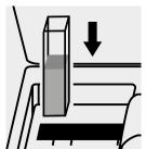
Place the cell into the cell compartment.
