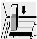
Place the cell into the cell compartment.
