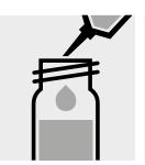
Pipette 0.50 ml of the sample into a reaction cell, close with the screw cap, and mix.
