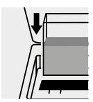
Place the cell into the cell compartment.
