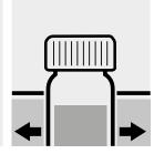
Temper the test tube in a water bath at 40 °C for 5 minutes.
