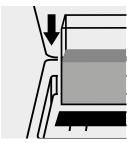
Place the cell into the cell compartment.
