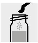
Add 1 level green microspoon of **Ph-2K**, close the cell with the screw cap.
