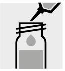
Add 3.0 ml of the sample with pipette, close the cell with the screw cap, and mix. Caution, cell becomes hot!
