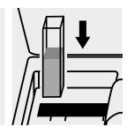
Place the cell into the cell compartment.
