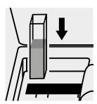
Place the **cell A** into the cell compartment. The measurement is performed automatically.
