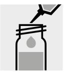
Add 1.5 ml of **B-2** with pipette and close with the screw cap.
