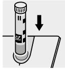
Place the **cell PO<sub>4</sub>-P** into the cell compartment. The results A ( $\Sigma$  P), Align the mark on the cell B (PO<sub>4</sub>-P), and C (P<sub>org</sub>) with that on the photometer.
