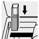
Place the cell into the cell compartment.
