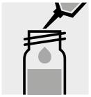
Pipette 1.0 ml of pretreated sample into a test acid. tube with screw cap.
