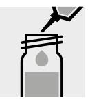
Add 0.25 ml of **Cl-1K** with pipette, close with the screw cap, and mix.
