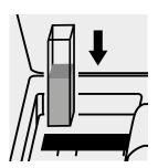
Place the cell into the cell compartment.
