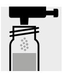
Add 1 dose of **P-1K** using the green dosemetering cap, close the cell with the screw cap.
