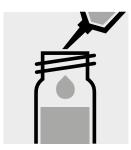
Pipette 1.0 ml of NO<sub>3</sub>-1K into a reaction cell, do not mix.
