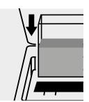
Transfer the solution into Place the cell into the cell compartment. The measurement is performed automatically.
