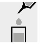
Transfer the solution into Select method no. 2503. the quartz cell.
