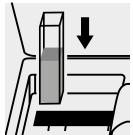
Place the cell into the cell compartment.
