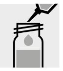
Add 2.0 ml of the sample with pipette, close the cell with the screw cap, and mix.
