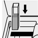
Place the cell into the cell compartment.
