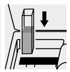
Place the cell into the cell compartment.
