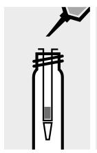
Run 3 separate 1-ml portions of **AOX-2** through the column. Discard the wash solution
