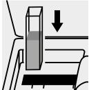
Place the cell into the cell compartment.
