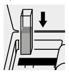
Place the cell into the cell compartment.
