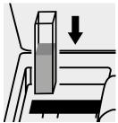
Transfer the solution into Place the cell into the cell compartment. The measurement is performed automatically.
