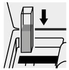
Place the cell into the cell compartment.
