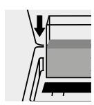
Insert the cell containing the sample into the cell compartment.
