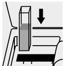
Place the cell into the cell compartment.
