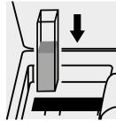
Place the cell into the cell compartment.
