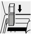
Place the cell into the cell compartment.
