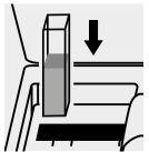
Place the cell into the cell compartment.
