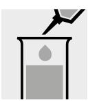
Add 0.10 ml of **reagent 1** with pipette and mix.
