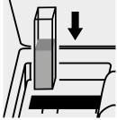
Place the cell into the cell compartment.
