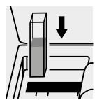
Place the cell into the cell compartment.
