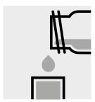
Transfer the solution into a rectangular cell.
