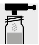
Add 1 dose of **Fe-1K** using the blue dosemetering cap, close the reaction cell with the screw cap.
