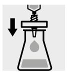
Filter or centrifuge turbid samples.
