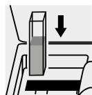
Place the cell into the cell compartment.
