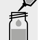
Add 2.0 ml of ethylene glycol monomethyl ether, close the test tube with the screw cap, and mix.
