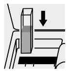
Place the cell into the cell compartment.
