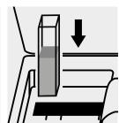
Place the cell into the cell compartment.
