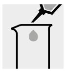
Place 20 ml of distilled water (Water Ultrapur, Cat.No. 1.01262, is recommended) into a second plastic vessel. (Blank)
