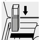
Place the cell into the cell compartment.
