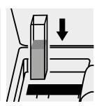
Place the cell into the cell compartment.
