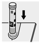
Place the cell into the cell compartment. Align the mark on the cell with that on the photometer.
