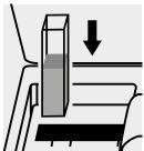
Place the cell into the cell compartment.
