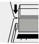
Place the cell into the cell compartment.
