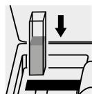
Place the cell into the cell compartment.
