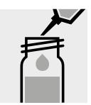
Pipette 6.0 ml of the sample into a reaction cell, close with the screw cap, and mix.
