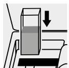
Place the cell into the cell compartment.
