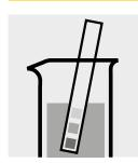
Check the pH of the sample, specified range: pH 0 - 10. If required, add dilute sulfuric acid drop by drop to adjust the pH.
