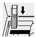
Place the cell into the cell compartment.
