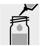
Pipette 2.5 ml of the sample into a test tube with screw cap.
