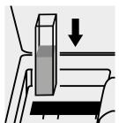
Place the cell into the cell compartment.
