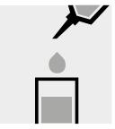
Transfer the solution into the quartz cell.
