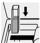
Place the cell into the cell compartment.
