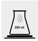
Weigh 50.0 ± 0.1 q of homogenized sample into a 250-ml conical flask.
