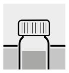
Temper the vessel in a water bath at  $95 \pm 5$  °C for **exactly** 10 minutes.
