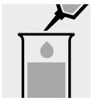
Add 0.60 ml of **NH<sub>4</sub>-1** (from Spectroquant® Ammonium Test, Cat. No. 1.14752) with pipette and mix.
