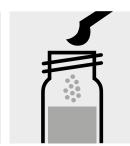
Add 1 level grey microspoon of Zn-5, close the test tube with the screw cap, and dissolve the solid substance.
