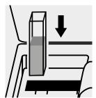
Place the cell into the cell compartment.
