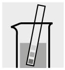
Check the pH, specified range: pH 2.0 – 2.5. If required, add dilute sodium hydroxide solution or sulfuric acid drop by drop to adjust the pH.
