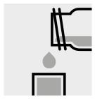
Transfer the solution into a 50-mm cell.
