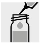
Add 2.0 ml of the sample-reagent mixture with pipette, close the cell with the screw cap, and mix.
