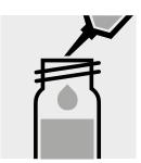
Add 2 ml of **color reagent**, close the test tube with the screw cap, and mix.
