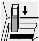
Place the cell into the cell compartment.
