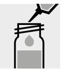
Add 0.50 ml of NO<sub>3</sub>-2 with pipette, close the cell with the screw cap, and mix. Caution, cell becomes hot!
