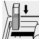
Place the cell into the cell compartment.
