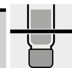
Remove the cell from the thermoreactor and let it, **standing on its head**, to cool for 1 hour.
