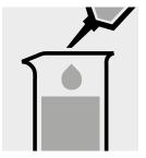
Add 1 ml of hydrochloric acid 1mol/l Titripur® (Cat. No. 1.09057) with pipette and mix.
