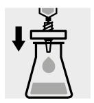
Filter or centrifuge turbid samples.
