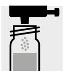
Add 1 dose of P-3K using the blue dosemetering cap, close the cell with the screw cap.
