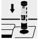
Select method with AutoSelector measuring range 1.0 – 15.0 mg/l Ca.
