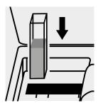
Place the cell into the cell compartment.
