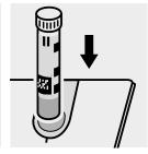
Place the cell into the cell compartment. Align the mark on the cell with that on the photometer. The measurement is performed automatically. **= cell A**
