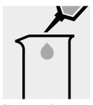
Place 50 ml of sample into a glass vessel.
