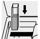
Place the cell into the cell compartment.
