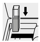
Place the cell into the cell compartment.
