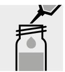
Add 2.0 ml of ninhydrin solution, close the test tube with the screw cap, and mix.
