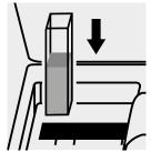
Place the cell into the cell compartment.
