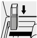
Place the cell into the cell compartment.
