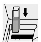
Place the cell into the cell compartment.
