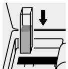
Place the cell into the cell compartment.
