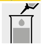
Pipette 0.10 ml of the sample into a test tube.
