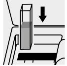
Place the cell into the cell compartment.
