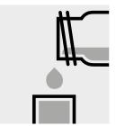
Transfer the solution into a rectangular cell.
