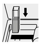
Place the cell into the cell compartment.
