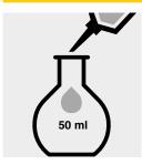
Place 20 ml of sulfuric acid 0.05 mol/l into a 50-ml volumetric flask.
