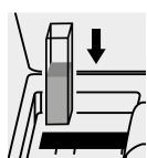
Place the cell into the cell compartment.
